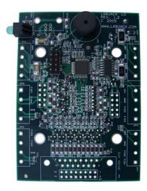
In the picture, note the holes available for 0.1" pin-header connectors. Connectors J3 & J4 provide pin-header access to the connections that would normally appear on the left and right screw-terminals. Connector J2 provides a pin-header alternative to the DB15 connector. The idea is that an OEM can connect ribbon cables to the pin-headers, or even plug the U3 directly to the customers main board designed with mating pin-header receptacles. See Appendix B for connector coordinates on the PCB.
