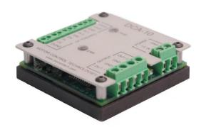
Every DCA-10 comes assemble with a sturdy anodized aluminum heat sink and enclosure. The integrated heat sink eliminates the need for additional heat sinking hardware. A small physical footprint (2.38" x 2.38" x 0.80") makes this unit easy to mount in the tightest of locations.
